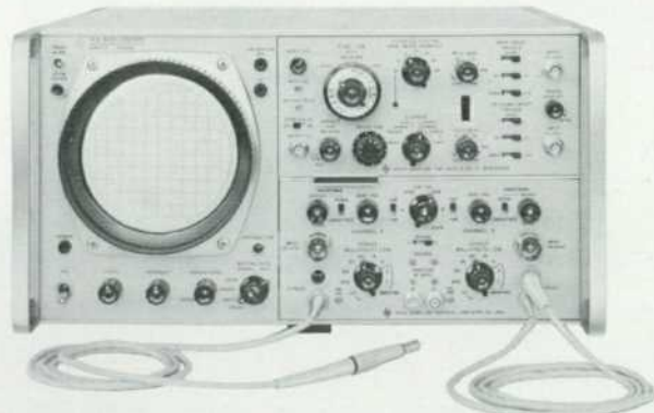
Fig. 2. Model 1425A Sampling Time Base and Delay Generator and Model 1410A 1-GHz Sampling Vertical Amplifier installed in Model 141A Variable Persistence Oscilloscope. Sampling gates in 1-GHz vertical amplifier are in probes. GR874 50Ω inputs lead to internal delay lines and trigger amplifiers for internal triggering.
