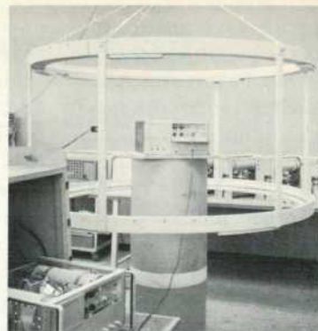
Fig. 6. Early production -hp- Model 5060A Cesium-Beam Frequency Standards were required to operate within specifications while subjected to magnetic fields up to two gauss in all orientations. Helmholtz coil was constructed to produce fields for test. Portable standard has also passed MIL-E-16400F shake and vibration test (MIL-STD-167), and exceeds the EMC (RFI) requirements of MIL-I-6181D. Production units are temperature cycled from -5^{\circ}\text{C} to +55^{\circ}\text{C} (operating) and are operated continuously for 15 days or more before being released.
